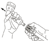
2 Slide down blue sleeve to release quick connect from the nozzle.
