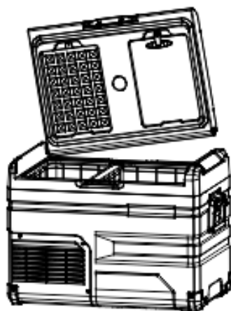
Align the door shaft with the hole on one side and insert it
