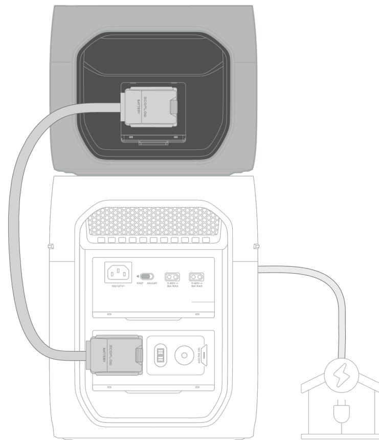
2. Once the battery is connected to the power station, turning on or off either one will activate or deactivate the other accordingly.
